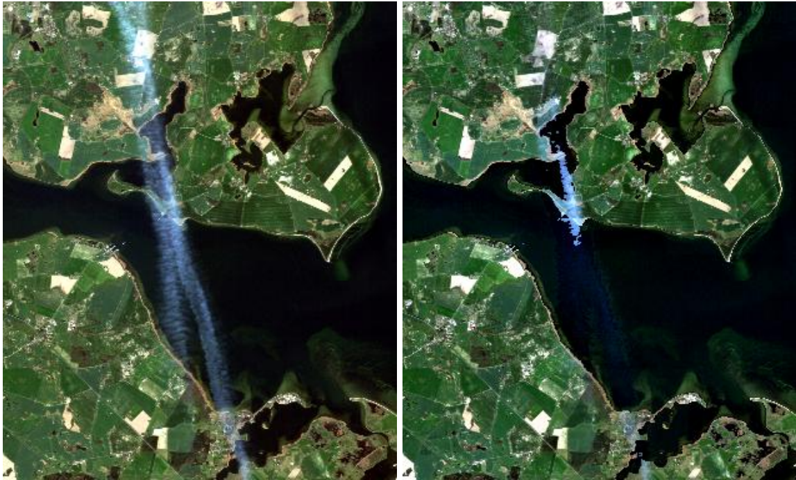
Figure 2.20: Haze removal over water, ALOS-AVNIR2 true color image, northern Germany, 16 April 2007. Left: part of original scene, right: after haze removal.
