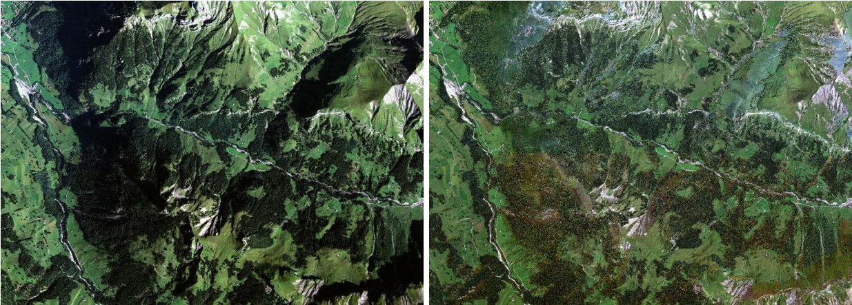
Figure 2.8: Effect of combined topographic / cast shadow correction: left: original RGB image; right: corrected image (data source: Leica ADS, central Switzerland 2008, courtesy of swisstopo).
